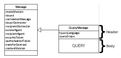
Figure 8: Information model components during a query
