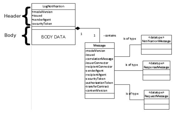
Figure 7: LogNotification with Body and Header
