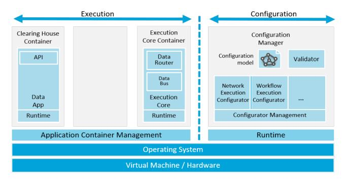
Figure 10: Relationship of IDS Connector and IDS Clearing House Container
