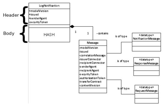
Figure 6: LogNotification Header and with Hash value
