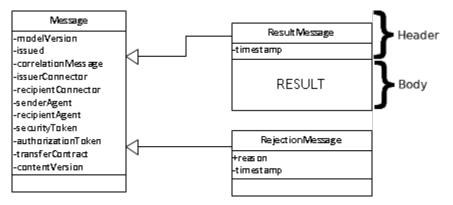
Figure 9: Information model components during a response
