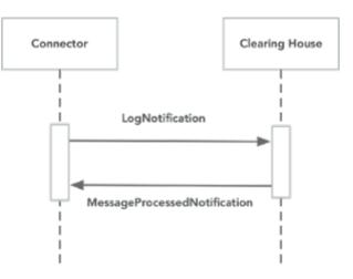
Figure 2: IDS Clearing House message logging process
