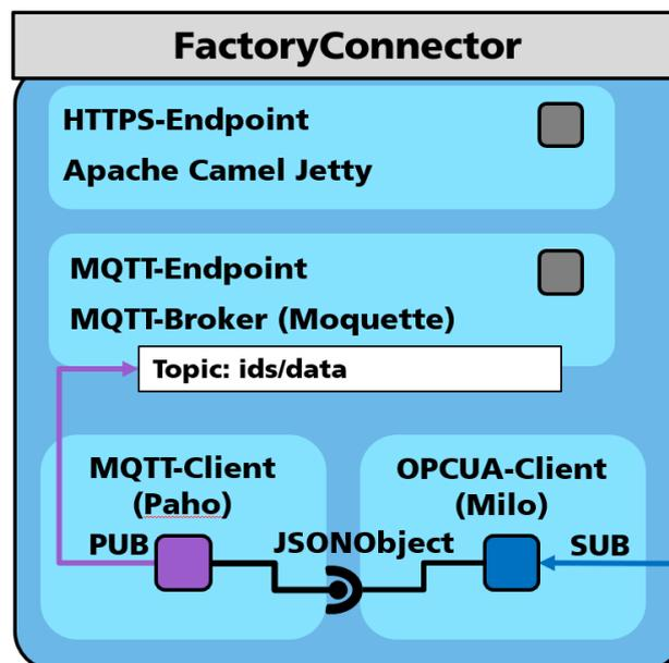
Figure 37: OPC UA-extended AASs and Base Connectors
