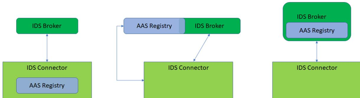
Figure 32: Various options for combining an AAS registry and an IDS metadata broker
