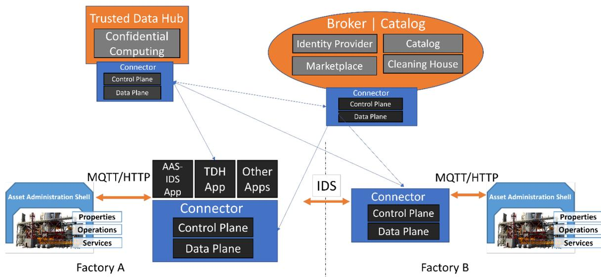
Figure 6: Toolchain Overview - Integration Eclipse BaSyx and IDS Connector
