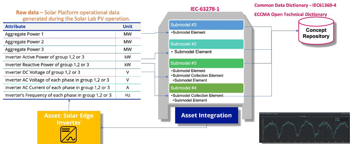
Figure 19: Connection between the AAS and the physical asset (Solar Edge inverter) [64]
