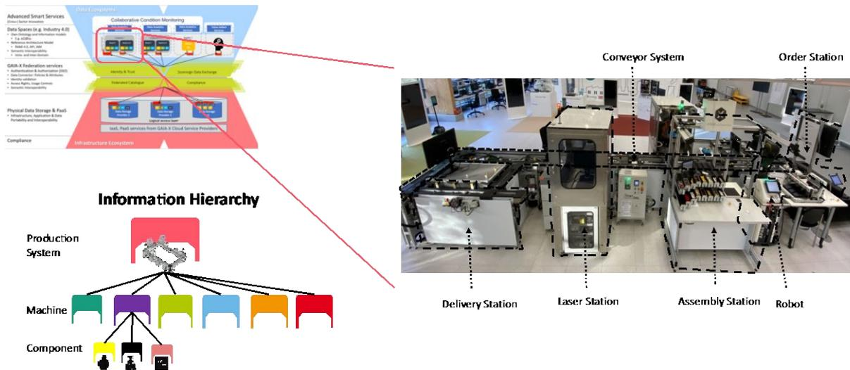
Figure 25: The location of the Customizable Production System (CPS) from SmartFactoryOWL in the architecture
