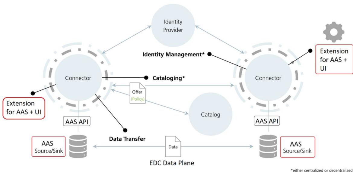
Figure 39: An approach for the integration between the AAS and the EDC connections
