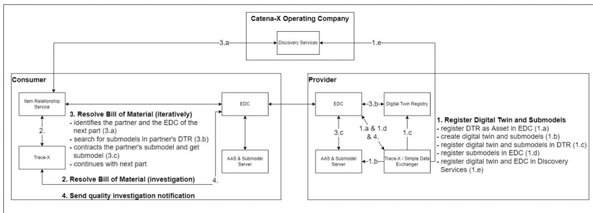
Figure 8: Simplified architecture of the Quality use case<sup>1</sup>
