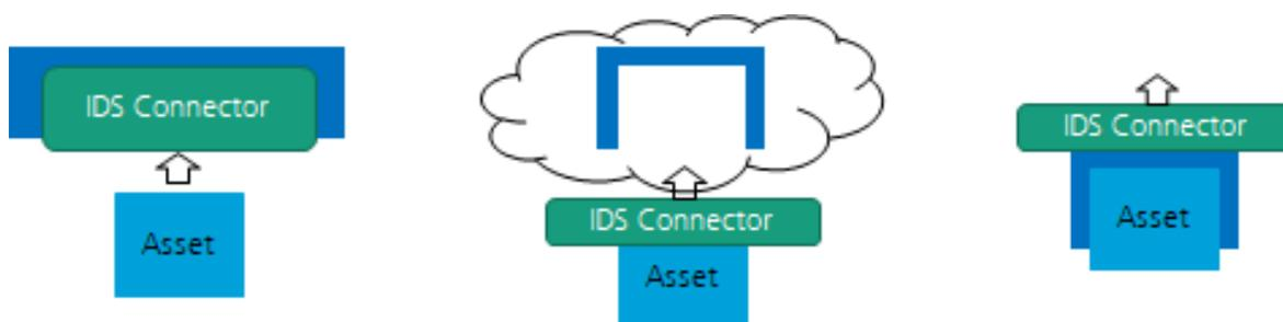
Figure 33: Options for integrating an IDS connection and an AAS
