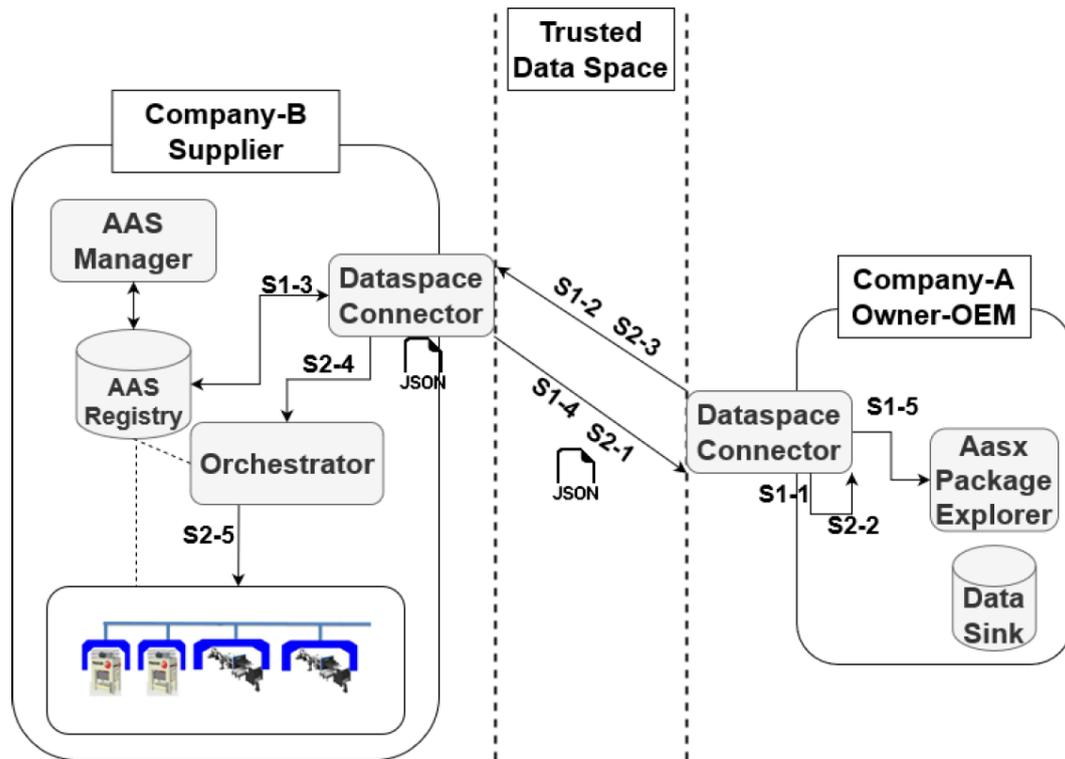
Figure 3: Data Sequences in the Use Case [10] Lessons learned from the joint use I4.0 & IDS concepts/components and recommendations for improvements
