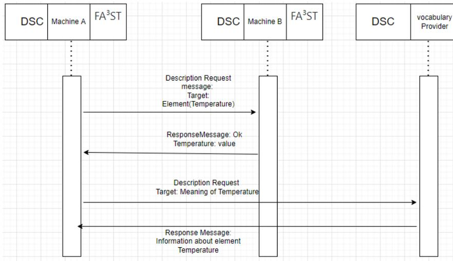
Figure 41: Use case „Collaborative Condition Monitoring“
