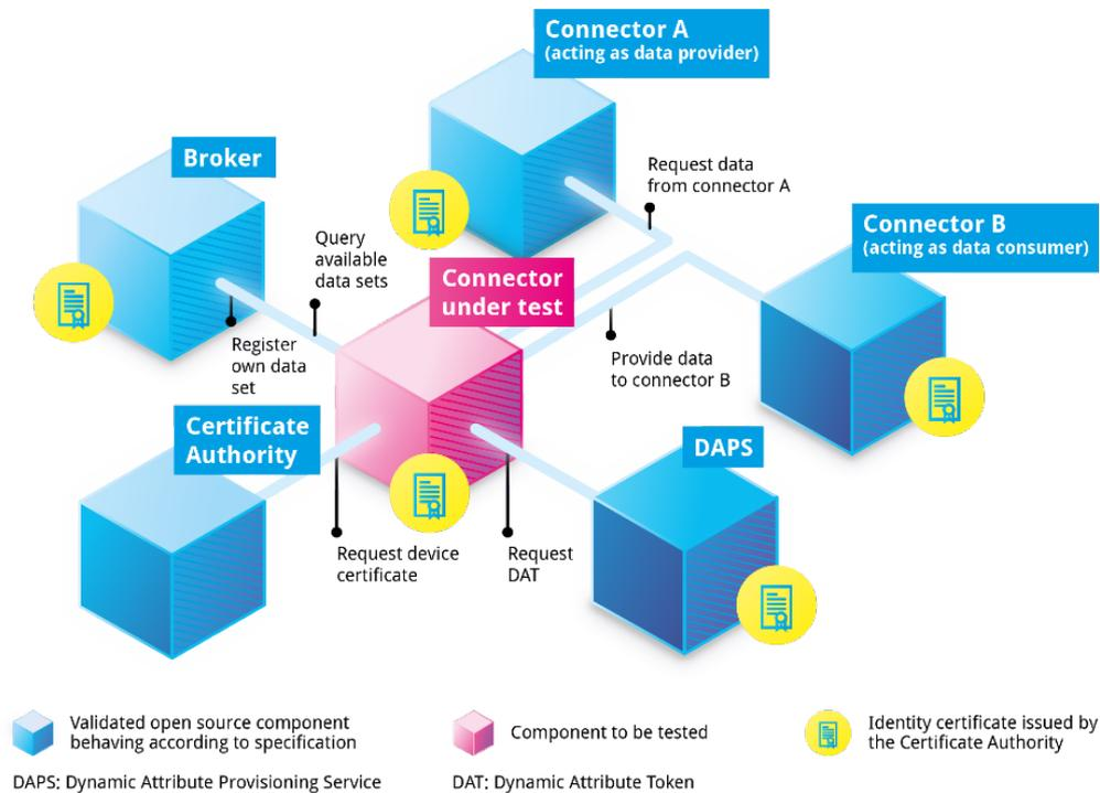
Figure 4: IDS testbed components [13]
