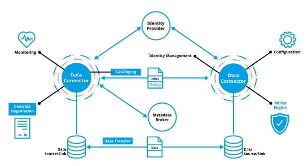
Figure 2 Data Exchange Services realized by a data connector as described in the IDS-RAM section 3.5.2
