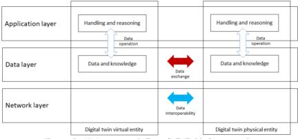
Figure 4 – HLA representation of digital twin example
