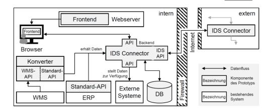
Figure 8 Technical architecture of the prototype (Opriel 2021). The grey boxes represent the components of the prototype; the white ones are the components of the legacy system; the arrows depict the data flow.
