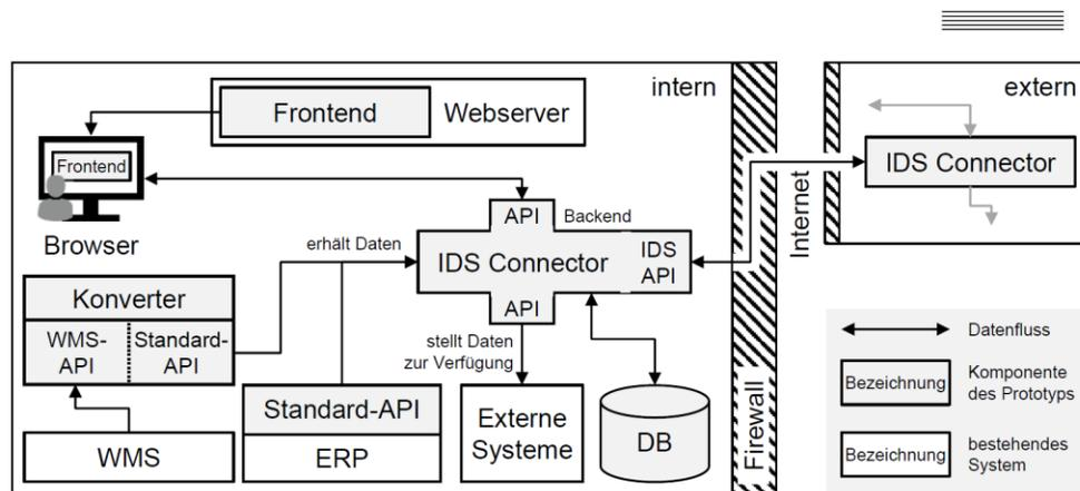
Figure 8 Technical architecture of the prototype (Opriel 2021). The grey boxes represent the components of the prototype; the white ones are the components of the legacy system; the arrows depict the data flow.
