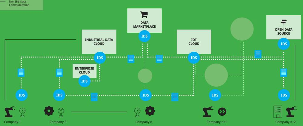
By proposing a specific software component, the International Data Spaces Connector, industrial data clouds, individual enterprise clouds, on-premise applications, and individual connected devices, can be connected.
