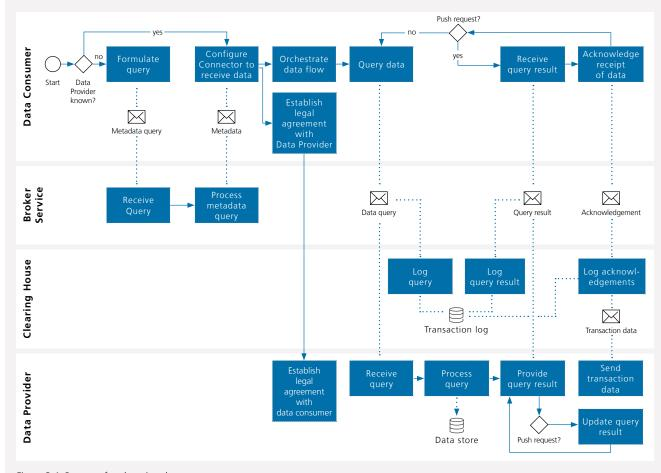
Figure 3.4: Process of exchanging data
