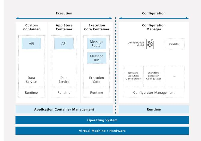
Figure 3.28: Reference Architecture of Connector
