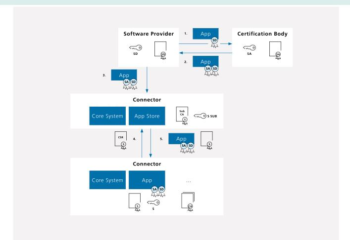
Figure 4.6: Software development, approval, and download process
