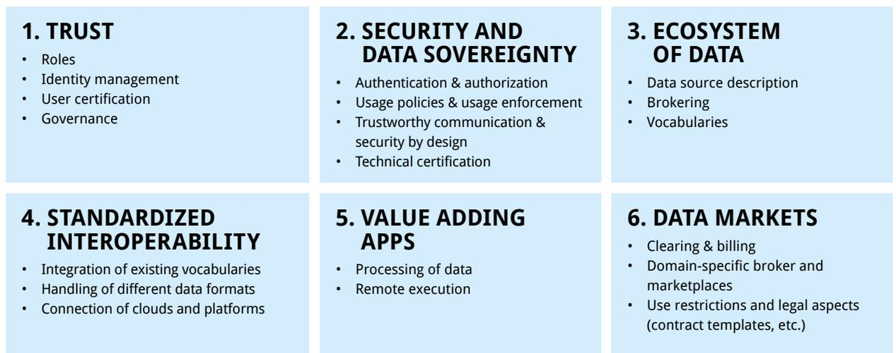
Figure 3.2: Functional architecture of the Industrial Data Space
