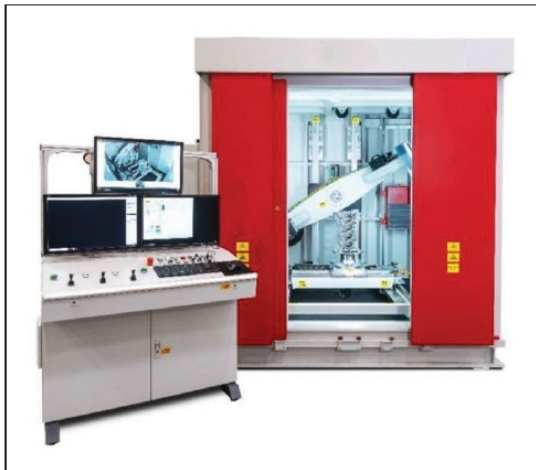
Figure 2. Typical example of an X-ray cabinet of the third industrial revolution, equipped with computer numerical control (CNC) drives.
