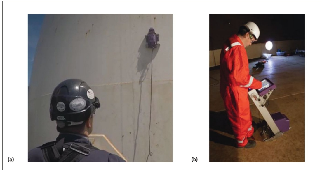
Figure 4. Nonintrusive tank inspection: (a) remote crawler utilizing dry-coupled UT; (b) MFL floor scanning for out-of-service tank.
