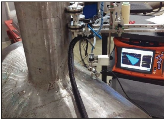
Figure 8. Nozzle inspection with a PAUT unit and specific scanners to hold the probe on the main pipe.
