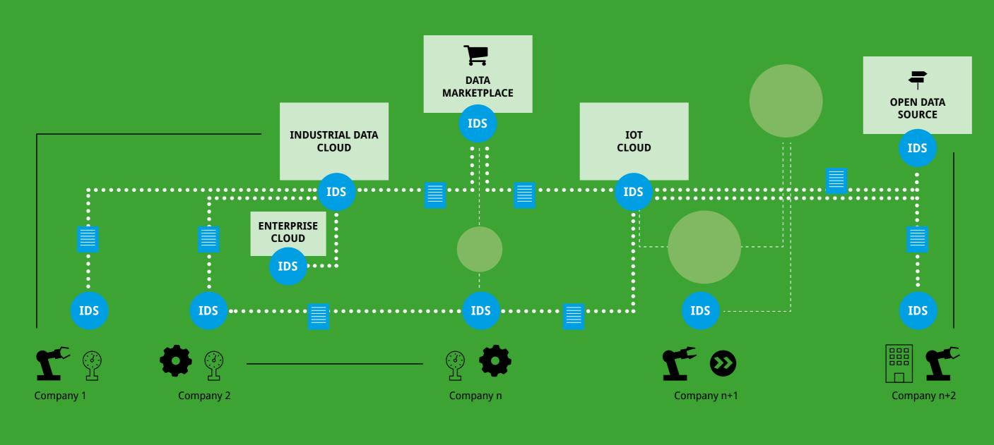
By proposing a specific software component, the INTERNATIONAL DATA SPACES Connector, industrial data clouds can be connected, as well as individual enterprise clouds and on-premise applications and individual connected devices.
